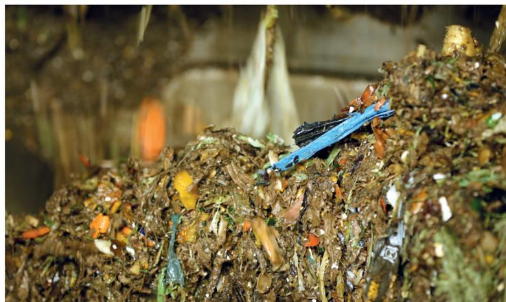
Separated contaminants consisting mainly of plastic- and carton packaging along with citrus peels coming out of the reject separator before going into the dewatering process. Notable is the intact "unmacerated" condition.
