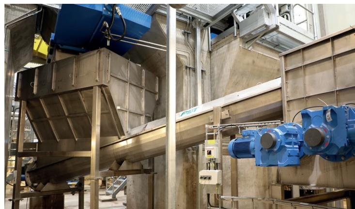
A receiving bin (left) under the reject separator takes the entire volume of purged reject. A PST screw conveyor feeds the reject in a metered fashion to the dewatering step for the rejected materials.
